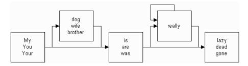
The set of sentences generated by this state machine is not finite because you can always follow the loop around "really" an infinite number of times. The notion that you can generate an infinite language with a finite generator or description is a crucial concept that you will see again.
