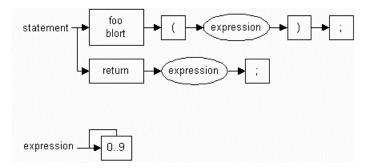
To distinguish between nodes that generate a word directly and invocations of submachines, use rectangular states for generators and oval states for submachine invocation states. Pushdown machines specified graphically in this manner are called *syntax diagrams*. The labels of the submachines correspond to the grouping constructs found in a sentence's tree structure representation. The sentence structure of "return 9;" in tree form looks like:
