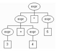
A machine, state or pushdown, that can generate a sentence in more than one way is an ambiguous language generator because it can mean two different things when generating the same sentence. In other words, if a machine can yield more than one tree structure for a given sentence, that machine is ambiguous as the sentence structure is ambiguous. Ambiguity is a problem because structure is the basis of meaning and leads to problems regardless of whether you are generating or recognizing sentences.
